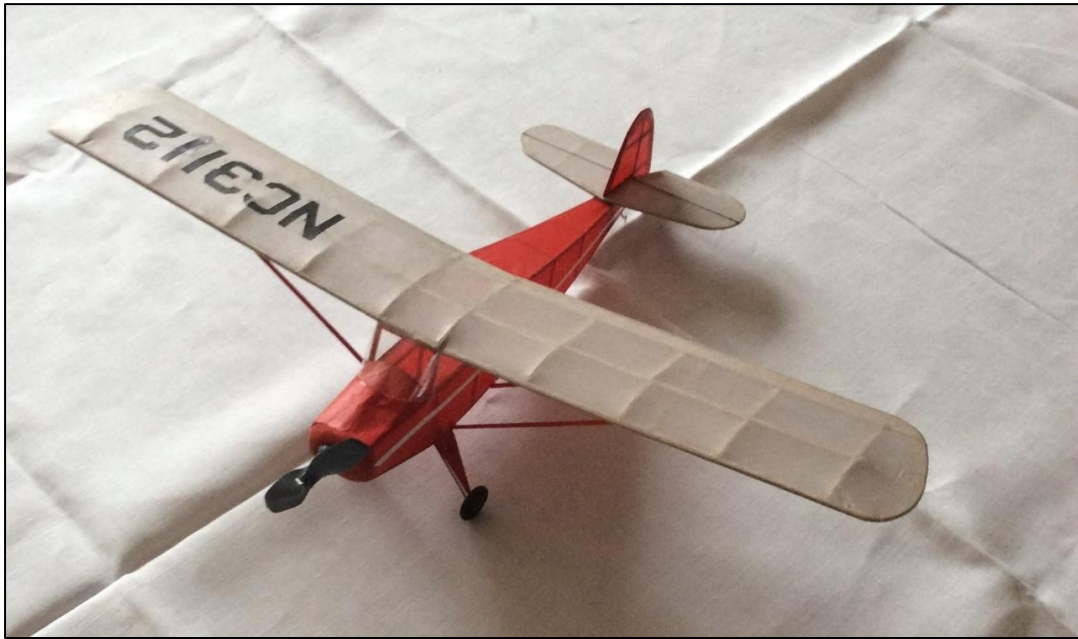
This is a Porterfield 65 Dime Scale from a Comet kit. Wingspan is 16", it has 32 square inches wing area and weighs 13.3g (0.47 oz) empty. Wing loading is 0.41 g/sq in, power is expected to be a 7" loop of 1/8".
