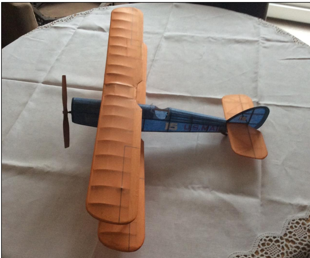
Airco D.H.4 built from a Comet kit. Span is 21 inches, wing area is a generous 115 sq inches so at 47.6 grams empty it has the same wing loading (0.41g/sq in) as the Porterfield! Power to begin with is expected to be an 11 inch loop of 1/8"
